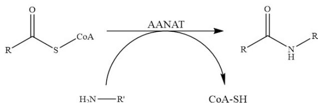
**Figure 1** Mechanism for the AANAT-catalyzed *N*-acetylation of amines and arylalkylamines.
