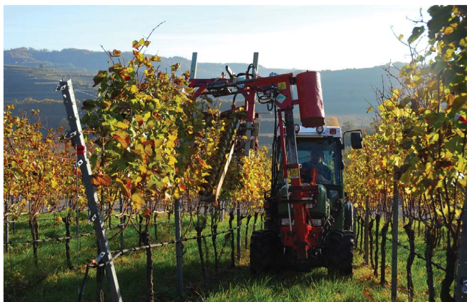
Figure 2 Commercially available vineyard cultivation machinery (ERO shoot binder) simultaneously modifiable for mechanical deployment of pheromone loaded mesofibers as well as weed control in South German vineyard of WBI Freiburg, Germany (photograph by M. Breuer).
